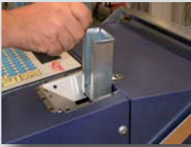
Interchangeable input hoppers for dog tags and medical alert tags for easy change
